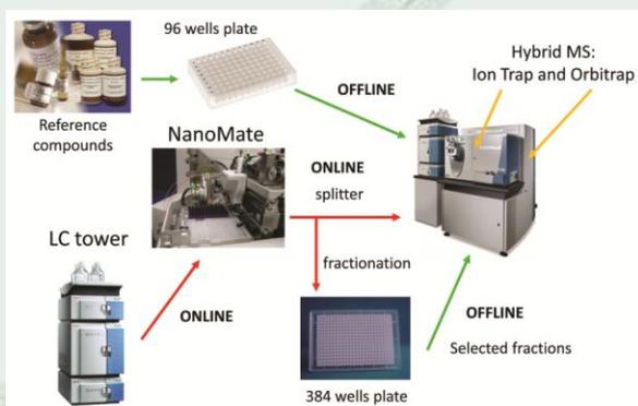
Figure 1: Schematic overview of MS<sup>n</sup> spectral tree data generation.
